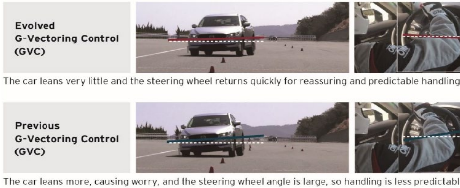
The car leans more, causing worry, and the steering wheel angle is large, so handling is less predictable
