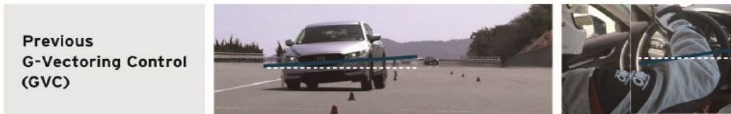
The car leans more, causing worry, and the steering wheel angle is large, so handling is less predictable
